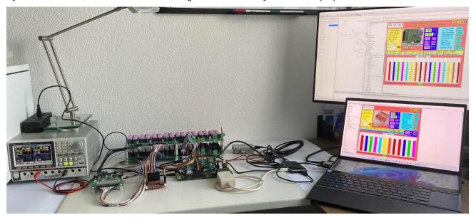
Figure 18: The full BMS setup using two battery boards with the mixed system of the TI bq76PL455EVM and the Infineon TLE9012AQU BMS boards connected to a single microcontroller while running two separate instances of Embed with both GUIs monitoring the system simultaneously. CAN bus and MOD bus interfaces are also connected.
